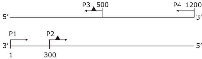
PCR was performed using primer pair P1 and P3 in one vial and P2 and P4 in another vial. The purified PCR products from the two vials were mixed and subjected to another round of PCR with primers P1 and P4. The final PCR product will correspond to a
